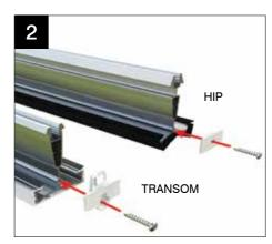
Attach the glazing bar end cap fixing blocks - as access restrictions may prevent easy fixing later. NOTE: These 'snap out' of the end caps when despatched from the factory.
