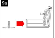
Remove any handling tape around the perimeter of the unit. Take care lowering the glazed unit into position on the internal lower muntin bar.
