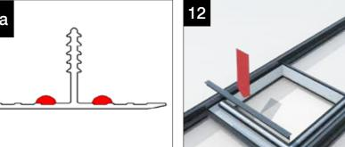
Locate the external lower muntin bar with the internal lower muntin bar, knock into place. The lower muntin may need supporting from underneath whilst secured into final postion.
