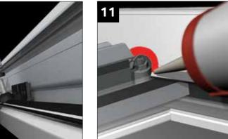
Seal around the notched hip bar top cap ready to receive the jack rafter capping.
