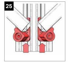
Ensure that glazing stops are pushed up the glazing bar and are firmly located against the glazing end profile. Please note the glazing end profile may be mitred in some cases.
