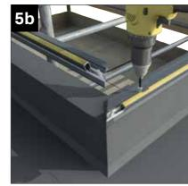
Check the required number of bolts are in the eaves beam/rail. Seal cut ends of eaves. Line up eaves along outer edge of kerb\* and screw down using appropriate 5mm x 50mm fixings (not supplied) ensuring good engagement.
