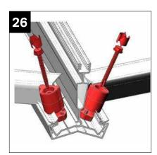
Ensure that the glazing end stops have been positioned correctly then screw down into the glazing bar, using the fixings provided. Now fully peel away protective film from glazing support at eaves and ridge and press glazing down firmly.
