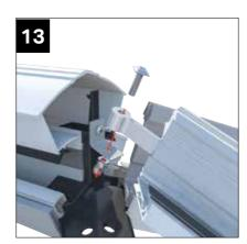
When a transom is fitted between hips, lift transom bar sleeved spiggot over bolt, then tighten nut.
