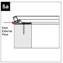
Aluminium eaves beam/rail (not the PVCu) sleeve) flush with external face of kerb.
