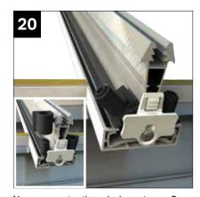
Now move to the glazing stage. Snap off appropriate handed glazing stop (LH shown). Handing marked at base of glazing stop. Line up the rounded edge on base plate next to central web of glazing bar and tuck under gasket side of bar. Rotate glazing stop into position. Push the grommet over the post. Slide assembly down to end of bar.
