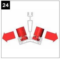
The glazing end stops fitted earlier should be pushed away from the centre of the bar and tucked under the gasket side of the glazing bar as shown. These are handed components, ensure they are positioned on the correct sides of the glazing bar.
