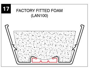
Ensure the foam does not interfere with the clips by pinching it towards the centre of the bar.
