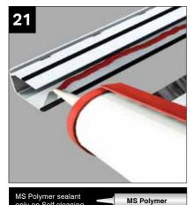
Seal underside of top face of glazing end profile as shown (PVCu version of end profile is shown - if aluminium glazing bar top caps, this end profile is also aluminium).
