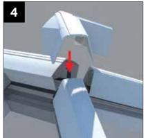
Press firmly down on the ridge end top cap until it clicks into position on the ridge end.
