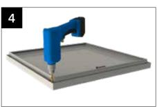
Finally re-fasten the factory fitted screws.
