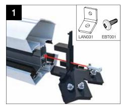
LANRF001 is supplied pre-installed into the bar. Remove and fix radius end (LAN032BL) then replace the screw. If using 3 bar attach LAN031 using EBT001.
