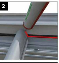
MS Polymer sealant only on Self cleaning glass
