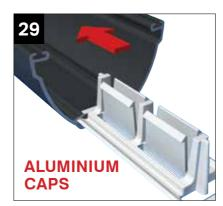
This stage should have been prepped in the factory. If not take the aluminium top caps and lay them onto a protected surface. Slide clips into each bar - position down from ridge / eaves at a max centre of 100mm and then at 500mm centres (max) inbetween.
