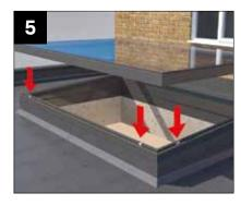
Fit the top glass frame onto the PVCu frame. Carefully lower into position and then apply downwards pressure to opposite sides to activate clips locking feature. (You will hear a click). NOTE: Larger units will require multiple persons to lift.
