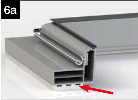
6a If existing glazing is 32/35mm a packer will have been pre-fitted to the frame.
