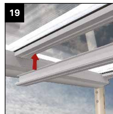
19 Complete the installation of the internal T sections.
