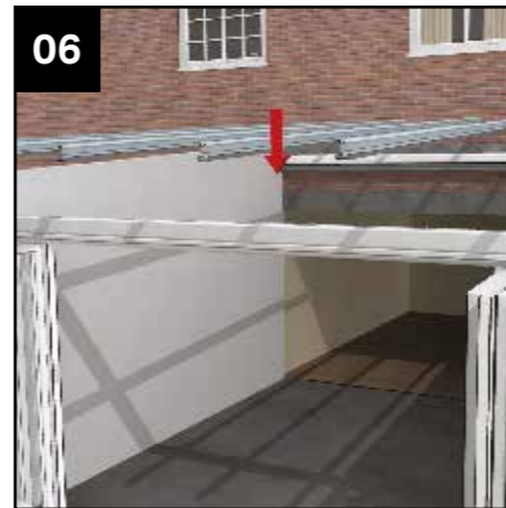
06 Next attach the Super Duty Eaves Beam to the head rail of the bi-fold doors. Lift the glazing bars into position and drop over the twin bolts in the captivated bolt slot at eaves and wallplate.
