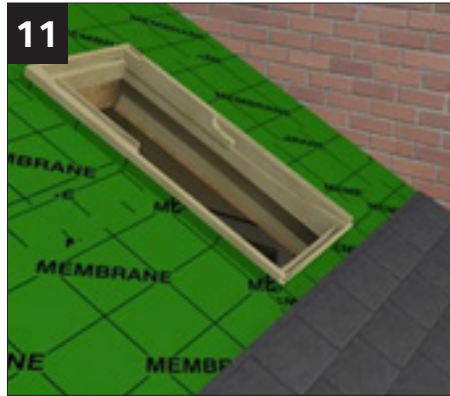
11 Install tiles up to the underside of the VELUX opening - refer to main guide to ensure correct tile spacing
