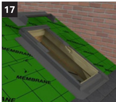
17 Fit the upper flashing panel
