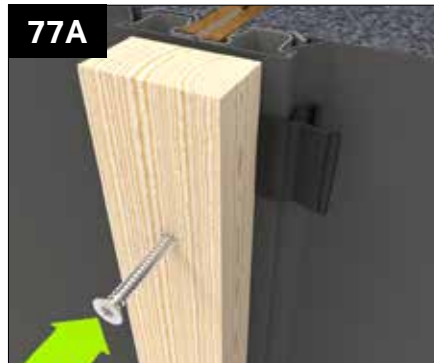
Position a 25mm batten, treated timber (optionally provided) or alternative, against the clips trapping the membrane in place. At apertures this batten is positioned in line with the opening as shown in image B. Secure the batten to the walling full and half clips at 450mm centres using the winged fixing screw (provided with battens). Please Note: - Excluding Flat Roof, the battens will be shorter than the clip length and should be set down from the eaves level or other air flow obstructing roof elements by 12mm to allow for ventilation.
