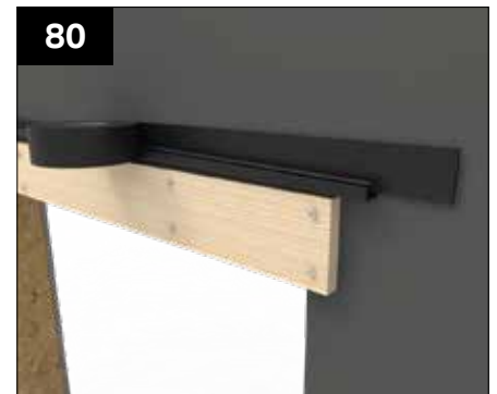
Using tape provided seal along the joint at the top between the soaker trim and the membrane.
