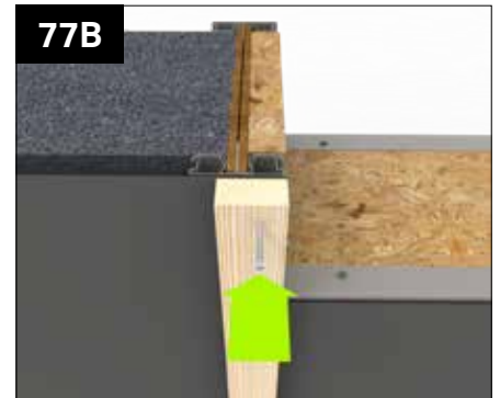
Position a 25mm batten, treated timber (optionally provided) or alternative, against the clips trapping the membrane in place. At apertures this batten is positioned in line with the opening as shown in image B. Secure the batten to the walling full and half clips at 450mm centres using the winged fixing screw (provided with battens). Please Note: - Excluding Flat Roof, the battens will be shorter than the clip length and should be set down from the eaves level or other air flow obstructing roof elements by 12mm to allow for ventilation.
