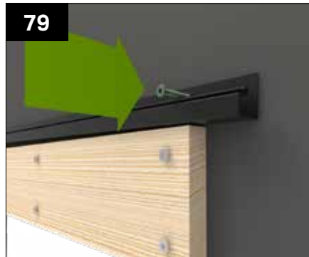
Fit the soaker trim to the wall at a slight angle using the GPHS fixing at 450mm centres, giving it a roughly one-degree fall. The battens should terminate above and below this trim.
