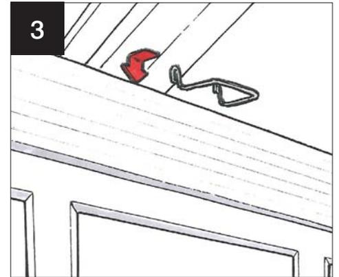
Over the 'V' groove fascia board at the eaves, at each transom bar position, hook over the cloaking panel support clips.
