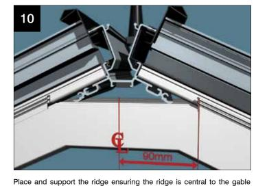
frame. Place the starter bar onto the firring top cap and secure to the ridge and eaves beam. Securely fix the starter bars to the gable window frame. Fit and glaze the roof in the normal manner.
