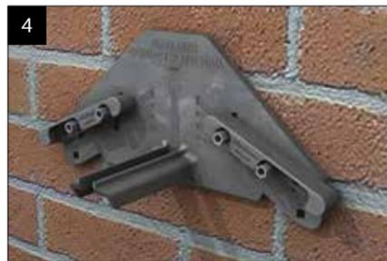
4 A 'Ridge Compression Plate' sits at the end of the aluminium ridge body where it joins the house wall - this distributes compression forces across the host wall and allows installers to assemble and suspend the starter bars prior to attaching the main ridge body.
