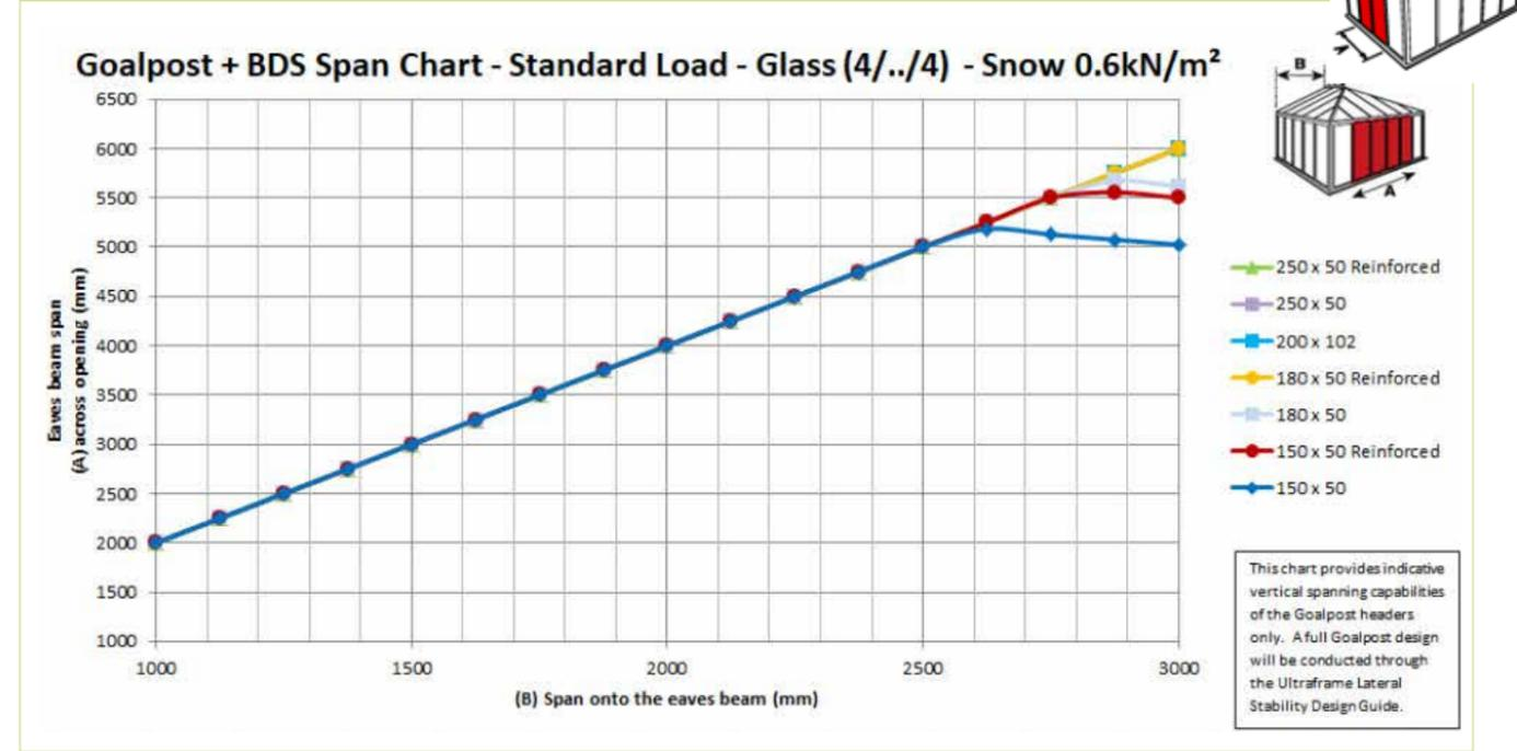
These span charts provide indicative vertical spanning capabilities of the Goalpost header beams only. A full Goalpost design will be conducted through the Ultraframe Lateral Stability Design Guide. They assume that there is no tie bar over an opening on Duopitch roofs.
