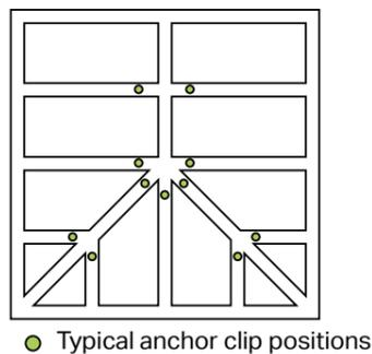
THE GLASS ROOF SYSTEM - GLAZING BARS
