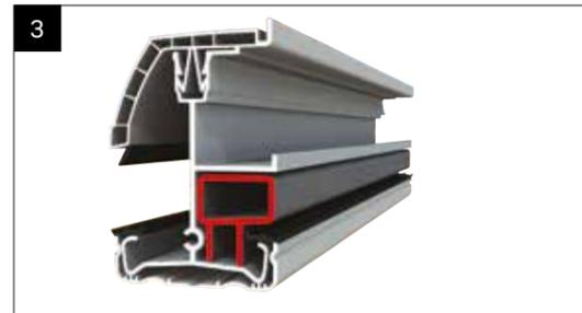
3 This short piece of reinforcement in each starter bar ensures that three anchor bolts are drilled into the host wall, when the reinforcement prevents the aluminium bar being crushed under excessive torque. It also ensures that additional reinforcement is offered where the bar intersects the eaves beam.
