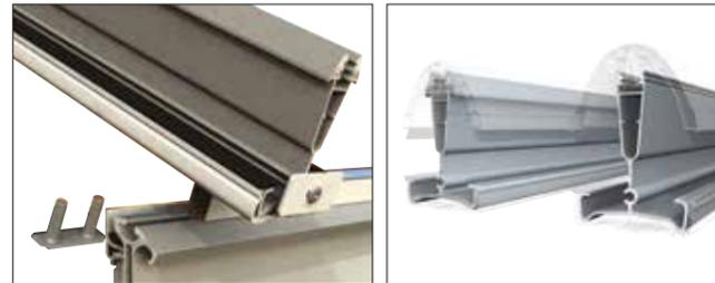
A twin bolt slides into the captivated bolt slot in the eaves beam, prior to the glazing bar being tightened down. Vic/Transom glazing bars come in heavy, medium and light versions
