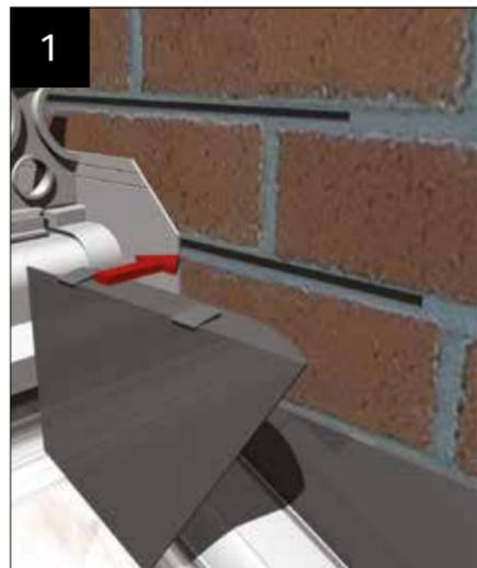
Apply 2 beads of silicone to integral weather-bars - insert into 35mm slot.
