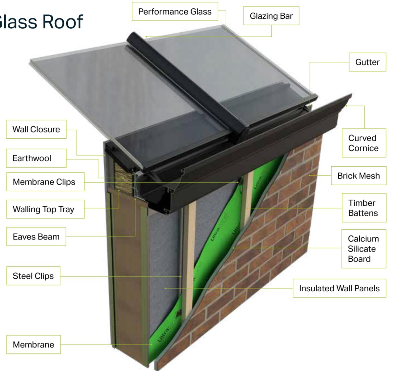
The Glass Roof is available with the hup! walling system from Ultraframe. The Glass Roof can be supplied with a hup! mini pelmet as shown below, or the internal pelmet can be widened to up to 1200mm making it the perfect place for spotlights or speakers.
