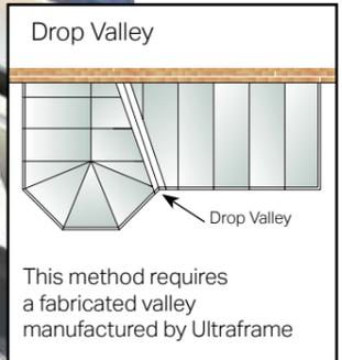
The Valley is a heavy weight structural component that drains two adjacent glazed roof slopes and connects to the eaves beam and the ridge/half ridge.
