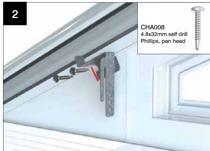
2 Take the gable bracket (CHA019R right hand shown). The back edge of the bracket should butt up to the pencil line. Align the top face of the gable bracket with underside of starter bar cladding.
