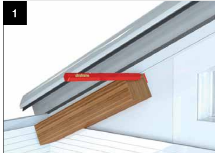
1 Using the location plan provided find the dimension for setting out the clip positions for the gable brackets. Measure up the bar from top edge of the fascia board and mark it.
