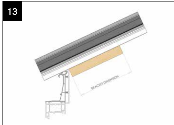
Measurements are ALWAYS from the top edge of the PFTB fascia board.
