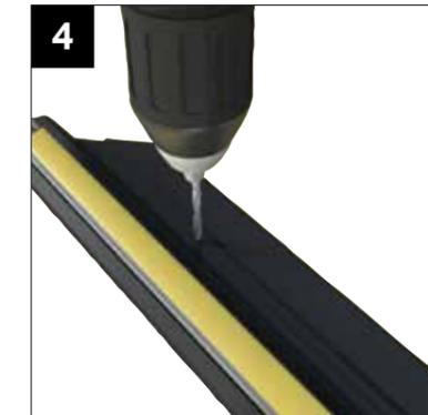
Pre drill 100mm from each end and drill a minimum of 4 holes at a max of 400mm centres using appropriate clearance drill. Now take the eaves beam/rail and ensure correct number of bolts are slotted into eaves beam/rail.
