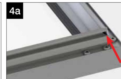
On the hinge side of the sash fill the hole shown above at either end with a blob of silicone.
