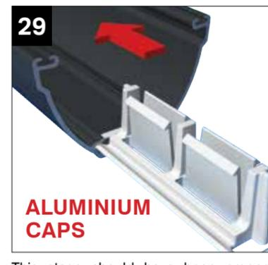
This stage should have been prepped in the factory. If not take the aluminium top caps and lay them onto a protected surface. Slide clips into each bar - position down from ridge / eaves at a max centre of 100mm and then at 500mm centres (max) inbetween.
