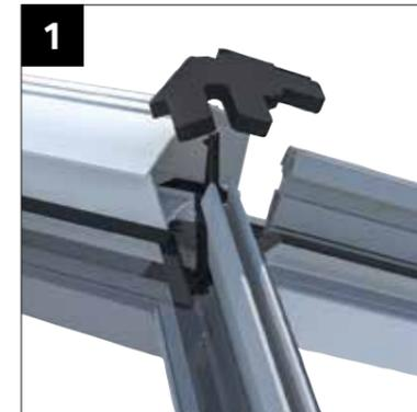
**ENSURE THE GLASS IS CLEAN AND DRY BEFORE FITTING.** Peel back protective film from weathering shield and position (adhesive face down) on glass, locating around the ridge and the hip bars. Press down firmly.
