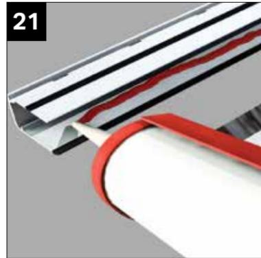
Seal underside of top face of glazing end profile as shown (PVCu version of end profile is shown - if aluminium glazing bar top caps, this end profile is also aluminium).
