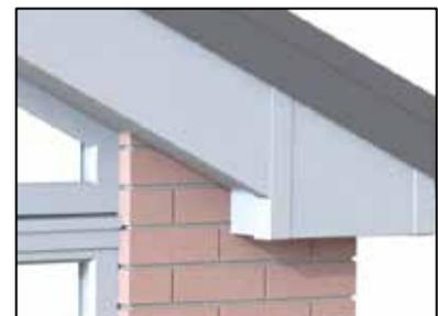
**Note: when Gable box is present, notching will be required to internal blockwork to accommodate.**
