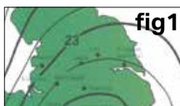
Use figure 1, page 42 to check the wind speed at the location (in this case its 23 m/s which translates on table 1 to 0.68 kN/m<sup>2</sup>). From figure 2, page 42 check the snow load at the location (which is 0.6kN/m<sup>2</sup>).
