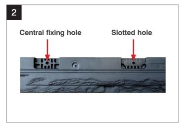
Fix through the central fixing hole for temporary fitting. (DO NOT FIX THROUGH SLOTTED HOLES UNTIL ALL STARTER STRIPS ARE IN PLACE)
