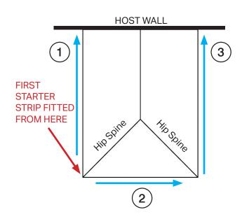
If a roof contains no rectangular glass panels and is classed as 'solid' then starter strips must be set out from the hip spine.
