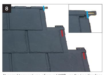
At normal temperatures, of around 15°C, use the insertion lines indicated red in the image. For low temperature installations, below 5°C, use the single insertion line indicated blue, at the top right of the tile.
