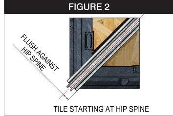
If the roof contains no rectangular glass panels, then the starter strips MUST be fitted at the hip spines first.
