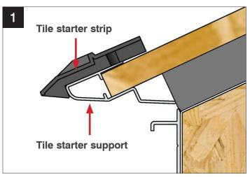
Place starter tile strip on starter tile support, make sure strip is a tight fit up against support.
