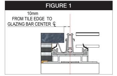
If the roof contains full rectangular glass panels, the starter strips MUST be fitted from the glazing bar.
