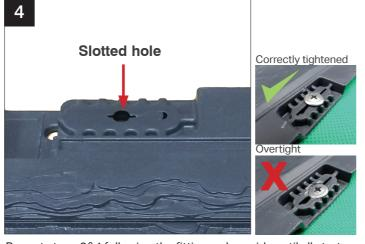
Repeat steps 3&4 following the fitting order guide until all starter strips are in place and are correctly fitted. Once correct, fully fix through slotted holes along the starter strips for permanent fix.
