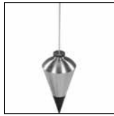
Plumb bob and string line
