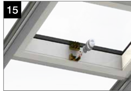
15 Align the winder bracket with bottom of vent frame (see section detail 15a for further information). Centrally align the winder bracket with the sash bracket. Once in position securely fit bracket in place using screws provided.
