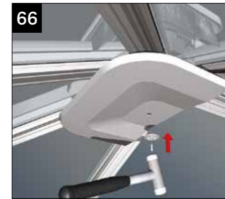
To fit the internal radius end capping insert the rose fixing button and tap the plastic rivet home to secure the button. On some occasions it may be preferable to test fit the ridge internal cladding prior to fitting the radius end capping.
