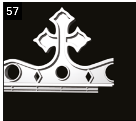
Cut back the underside of the last section of creasting by 40mm.
