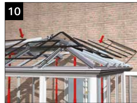
Glaze the lower pagoda roof fully.
