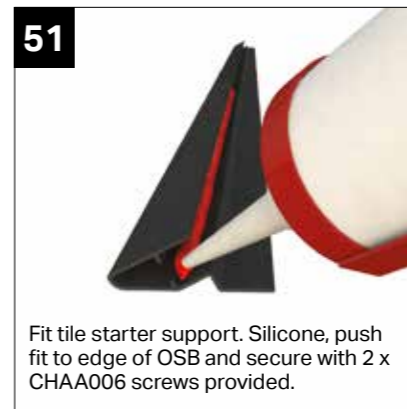
Fit tile starter support, silicone and screw fit. Using location plan, lift OSB board panel A into approximate position. Having fixed tile starter support onto end of OSB, place against ends of external panel clips to locate OSB. Locate first row of OSB panels around the roof using tile starter support to position. Work in the same order that the beams were put on (sides toward front)
