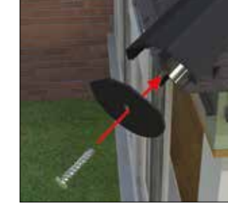
NRES 004 4.8 x 32 pan head self drill
