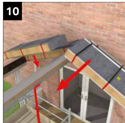
10 Continue fitting the panels from the host wall.
