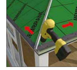
Fixing Ultratile starter strip
