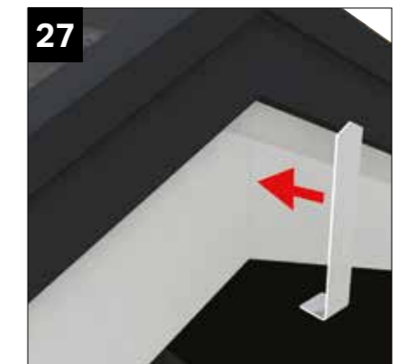
27 Fit the fascia ridge trim, modifying where necessary ensuring a neat finish.
