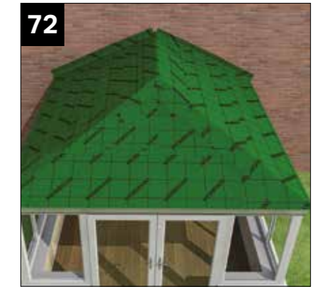
72 Image shows roof covered with breathable membrane. Follow the sequence. Membrane part no: RRMA050
