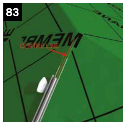
Place the hip spine with the centre aligned to the final point, mark each side of the spine then remove.
