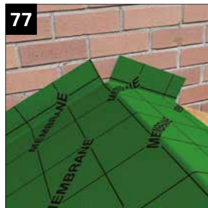
On solid roof, the membrane layer straddles the ridge. Slit as shown to allow transition to the opposite side. If the membrane falls short of the ridge plate, install an additional canopy, centrally over the ridge.
