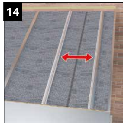
The expandable panel will expand sideways to take up any remaining gap.
