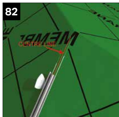
Find the centre line of the steel hip capping plate below the membrane and mark a centre line through to the final point.
