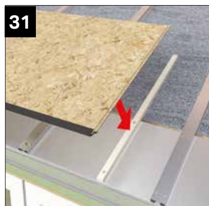
Where required support OSB board at butt joints using timber battens supplied. Battens are 65 x 19 x 700mm long (NRPB010). Only required over box beam. All OSB board edges are tongue and grooved to allow positive location. Continue to board from bottom to top (box beam to wall plate).
