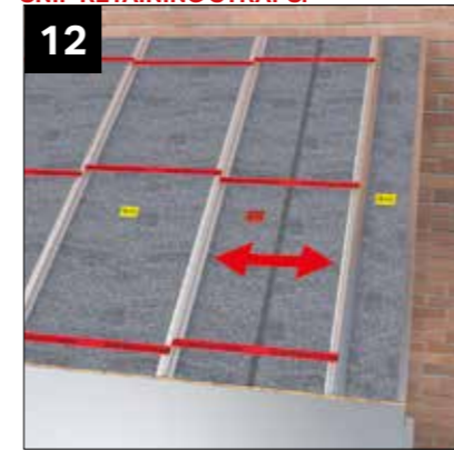
The red labelled panels are always installed last. DO NOT SNIP RETAINING STRAPS.
