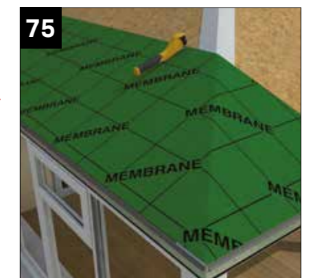
75 Minimum 200mm overlap over hips. Fix using staple hammer with maximum 12mm stainless steel staples. Take care not to cut through lower layers whilst trimming.
