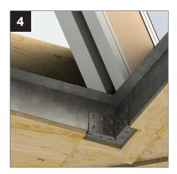
When in position, the hip should sit on the beam panel shelves as shown and be fixed as described in the main installation guide.
