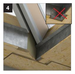
When in position, the offset hip wings should sit on the beam panel shelves as shown and be fixed as described in the main installation guide. NOTE: INTERNAL BEAM CORNER CLEATS NOT SUPPLIED IN VARIABLE PITCH SITUATIONS.
