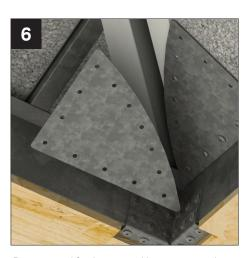
Position and fix the internal hip retaining plates using 18 x CHAA 006 screws provided.
