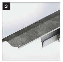
The hip assembly features a notched beam overhang and offset hip wings. The notch should be oriented towards the beam with the steeper pitch.
