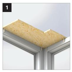
In variable pitch situations the beam setout shelf is asymmetric, with the longest side relating to the beam with the steepest pitch – see location plan.
