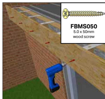
Fix through panel into fin temporarily using FBMS050 fixings.
