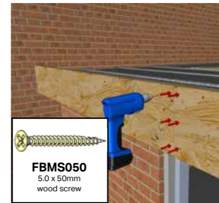
Once level, fix through the joint of the two panels using 6x FBMS050 fixings.
