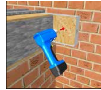
Secure through OSB fin into host wall
