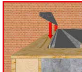
External panel clip running parallel to beam 1 per 300mm centres
