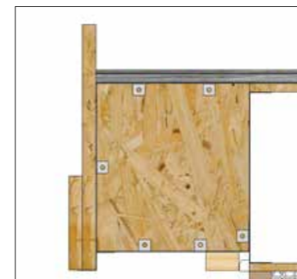
If you have an extended two tier cornice, the OSB fascia will look slightly different but the OSB fascia still sits on the Z section like above.
