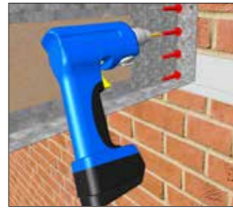
Intermediate beam to host wall Min 4 fixings per bracket
