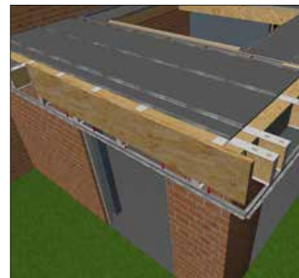
1a onto the Z section, start at the front left hand corner and align the end of the fascia to the end.
