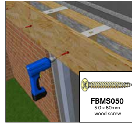
Clamp the fascia to the fin if possible, then temporarily fix into fins using FBMS050 until full elevation is in place.
