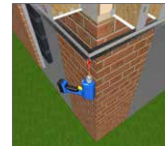
Connecting 2 x Z sections Pre drill and fix, 1 fixing per corner
