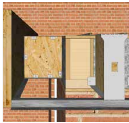
1a onto the Z section, start at the front left hand corner and align the end of the fascia to the end.
