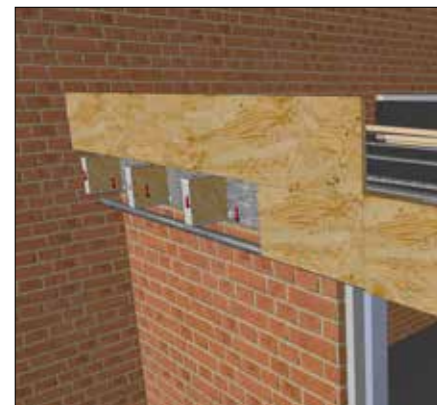
Place fascia panel 1b into place overlapping panel 1a.
