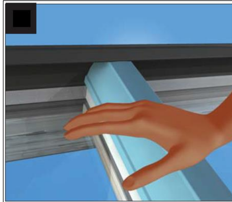
New Single Push Fit Top Capping Installation
