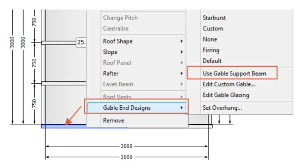
Once the GS has been applied you can then use the SDG to fix or you can apply manually by right clicking on the Gable End and then use the Eaves Beam menu.
