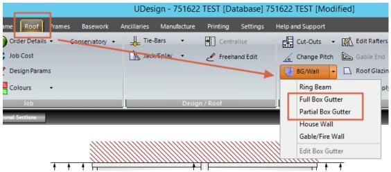
This box gutter only works with Heavy Eaves
