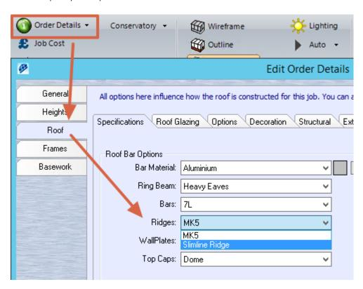
In the information window there is a message for Slimline Ridge, you can change to this ridge providing the pitch is  $25^\circ$
